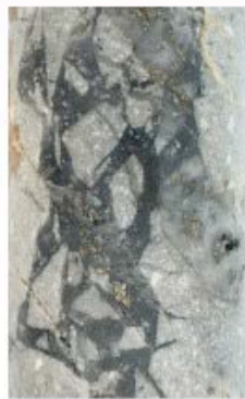
Drill core at RT-11 showing hydrothermal breccia with >0.5% Cu as chalcocite, which enables SXEW.
